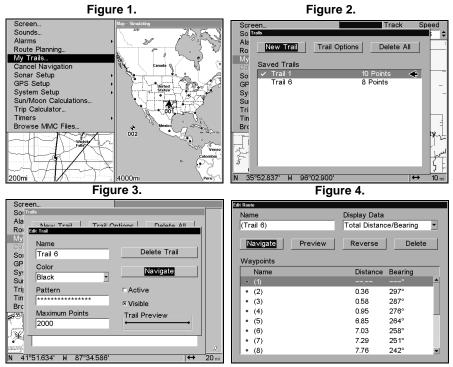
Navigate a trail menu sequence: Fig. 1, My Trails command. Fig. 2, Trails Menu. Fig. 3, Edit Trail Menu. Fig. 4, Edit Route Menu with Navigate command highlighted for Trail 6. A trail is always converted to a "route" when you navigate the trail. On the Map Page, a course line represents the trail you are navigating. The bearing arrow on the compass rose points to the next waypoint on the trail.
